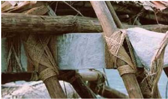
Seafaring in the Polynesian Outliers. Fig. 5 “Earth oven” and “fish eye” lashings on cross beams and outrigger struts of te puke canoe.
